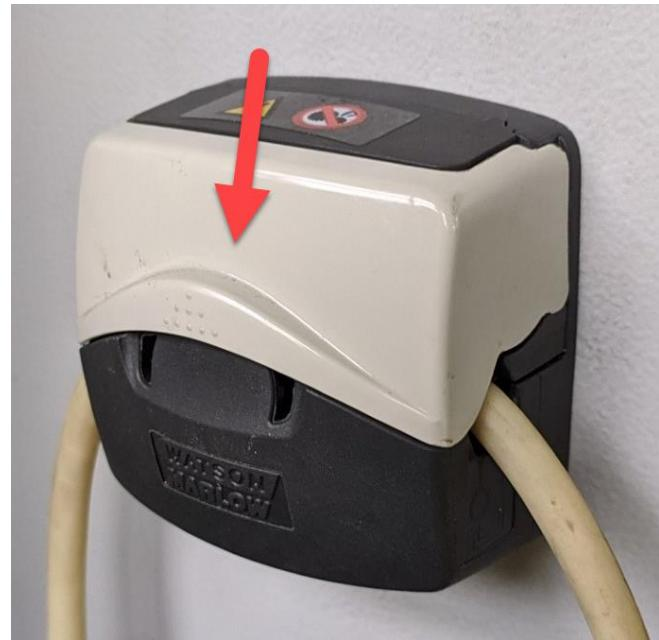
Remove old tube and install new tube
