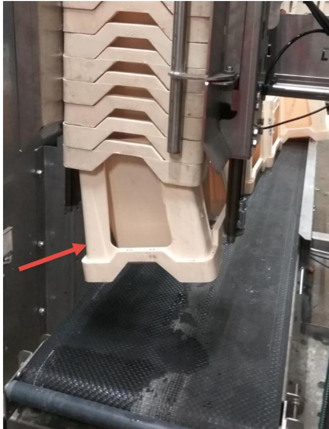
Remove bucket and press 'start' button. The lift is being reset when it's reaches the top position, then press start on the touchscreen.
